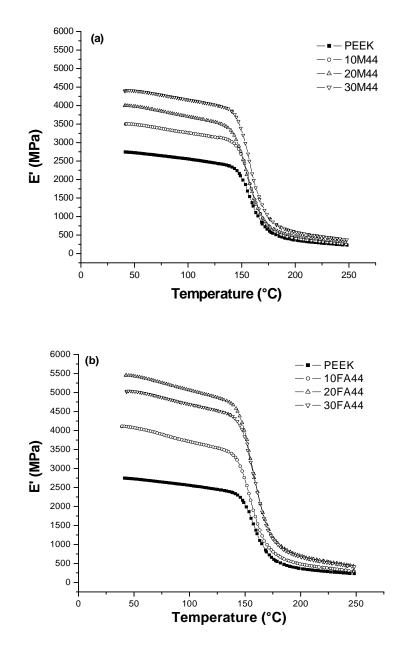
Figure 10. Dynamic mechanical spectrum of storage modulus of (a) PEEK mica composites and (b) PEEK fly ash composites.
