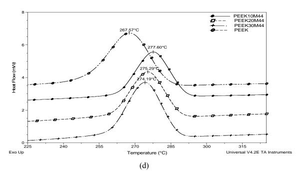
Figure 9. Modulated differential scanning calorimeter (MDSC) thermograms for (a) and (c) second heating curves of  $T_g$  and Tm of 44  $\mu$ m mica filled PEEK composites. (b) and (d) cooling curves of crystallization temperature Tc of 44  $\mu$ m mica filled PEEK composites.
