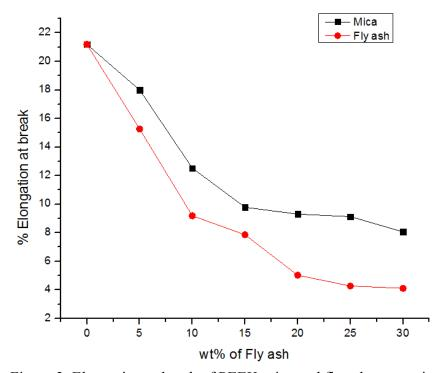
Figure 3. Elongation at break of PEEK mica and fly ash composites.
