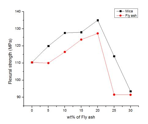
Figure 5. Flexural strength of PEEK mica and fly ash composites.
