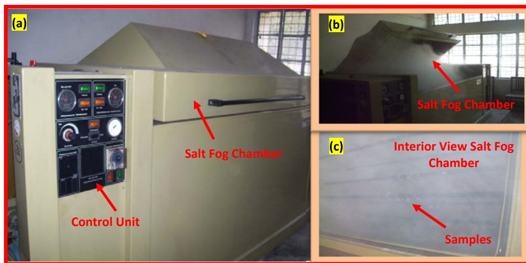
Figure 1. Experimental set-up for Salt spray (Fog) testing (a) Salt fog testing set up, (b) Salt fog chamber, (c) Interior view of chamber
