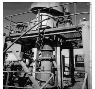
Figure 3. Yang jig plant installation.
