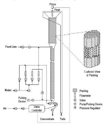
Figure 1. Yang jig Schematic Design.
