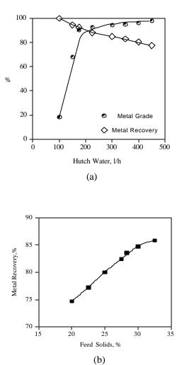
Figure 2. Effect of hutch water and feed solids on jig performance
