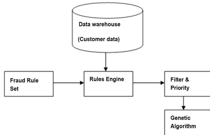
**Figure 3.** Implementation plan of genetic algorithm based system.
