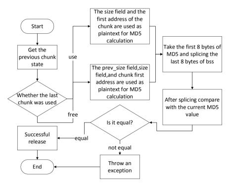
Figure 6. Free function release process.
