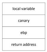
Figure 2. Chunk stack layout.
