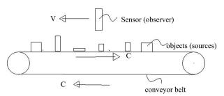
Figure 2. Sketch of a Conveyor Belt with a Doppler Shift.
