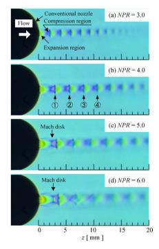
**Figure 8.** Schlieren pictures with vertical rainbow filter for conventional nozzle.
