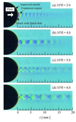
**Figure 10.** Schlieren pictures with vertical rainbow filter for improved nozzle.
