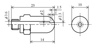
Figure 5. Improved leek peeler nozzle (dimensions in mm).
