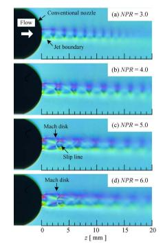
**Figure 7.** Schlieren pictures with horizontal rainbow filter for conventional nozzle.
