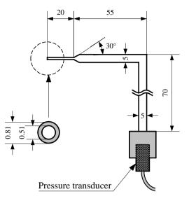
Figure 6. Schematic drawing of Pitot probe (dimensions in mm).
