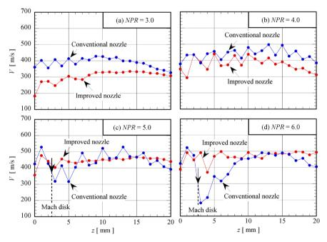
Figure 15. Centerline flow velocity distributions for conventional and improved nozzles.
