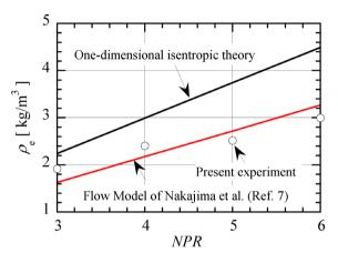
Figure 12. Comparison of theory with exit density of conventional nozzle.
