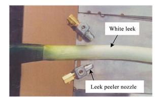
Figure 1. White leek on working bench with leek peeler nozzles.
