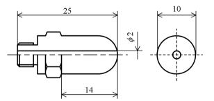
Figure 4. Conventional leek peeler nozzle (dimensions in mm).
