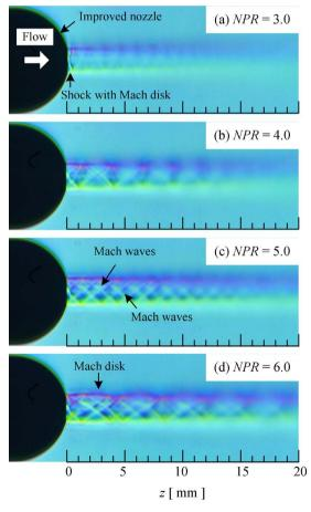
**Figure 9.** Schlieren pictures with horizontal rainbow filter for improved nozzle.
