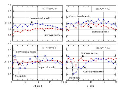
Figure 14. Centerline Mach number distributions for conventional and improved nozzles.
