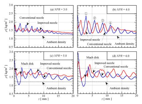
Figure 11. Centerline density distributions for conventional and improved nozzles.
