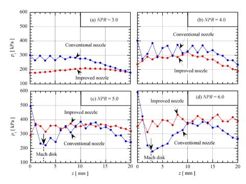
Figure 13. Centerline Pitot pressure distributions for conventional and improved nozzles.
