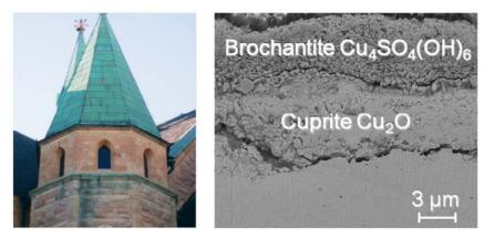
Figure 1. Green patina on a copper roof of a church in Stockholm, and released copper retained by the stone plinth beneath the roof (left). A cross section of a 350 year old naturally aged corroded copper roof with an outer green patina layer of basic copper sulfates and an inner brown layer of copper oxide (right).
