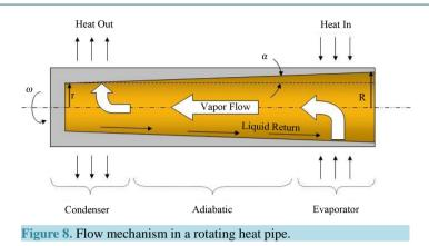
are insensitive to gravity, and will still operate when inverted, with the evaporator above the condenser. In this application, the vapor chamber acts as a heat flux transformer, cooling a high heat flux from an electronic chip or laser diode, and transforming it to a lower heat flux that can be removed by natural or forced convection.
