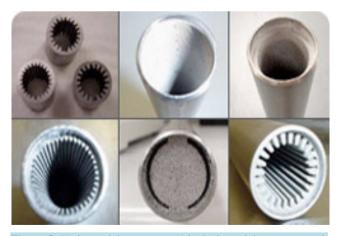
Figure 5. Various wicks structures (clockwise-axial grooves, mesh screen, sintered metal powders, sintered metal powder grooves) (fine grooves), sintered slabs, sintered metal powder grooves).
