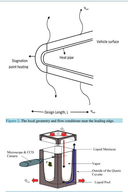
Figure 3. Constrained vapor bubble experiment for international space station.
