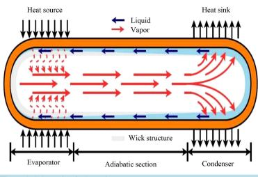
Figure 1. Schematic of a heat pipe.
