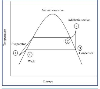
Figure 4. Thermodynamic operation of heat pipe.
