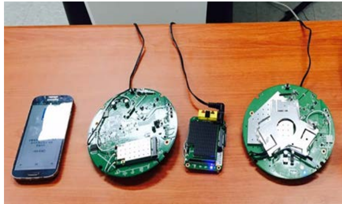
Figure 4. Wireless mesh network communication test.
