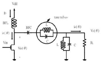
Figure 2. Novel design methodology schematic of class-F power amplifier.
