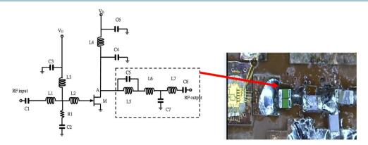
Figure 6. Output matching network of the class-F power amplifier.
