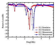
Figure 7. Return loss of the proposed class-F power amplifier.
