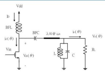
Figure 1. Original design methodology schematic of class-F power amplifier.
