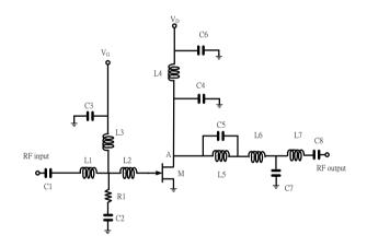
Figure 5. Schematic of the class-F power amplifier.
