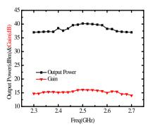
Figure 9. Saturation output power and gain as a function of frequency.
