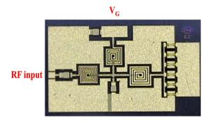
Figure 4. Chip photograph of the proposed PA.
