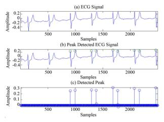
Figure 13. R peaks detection using ATV.
