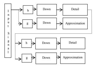
Figure 6. Filter bank tree decomposition.
