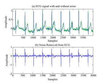
Figure 12. ECG signal before and after filtration.
