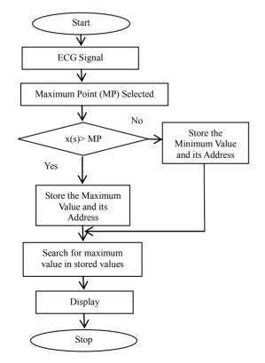
Figure 9. The flowchart of PPT.
