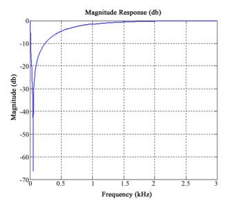
Figure 2. Frequency response of a 50 Hz NF.
