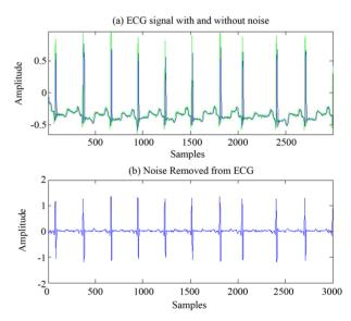
**Figure 10.** ECG signal before and after filtration (green color ECG signal with noise, blue color ECG signal after filtration).
