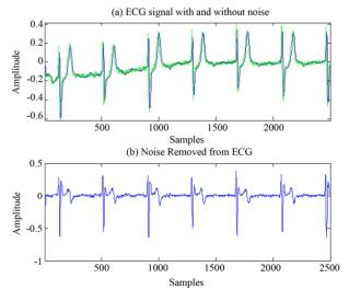
Figure 11. ECG signal before and after filtration.
