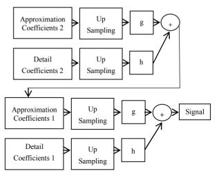
Figure 7. Filter bank tree reconstruction.
