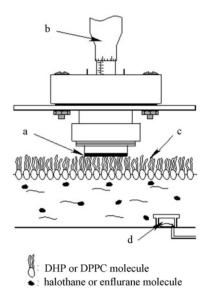
**Figure 2.** Schematic diagram of the central part of the QCM apparatus: a) QCO; b) micrometer; c) DHP or DPPC monolayer; d) small poly (tetrafluoroethylene) vessel and stirring bar.
