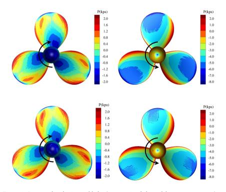
Figure 7. Pressure distribution on blades (top: restricted channel; bottom: open water).
