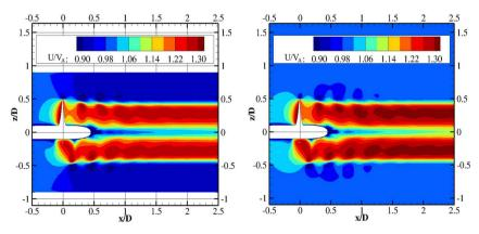
Figure 9. Axial velocity distribution (left: restricted channel; right: open water).
