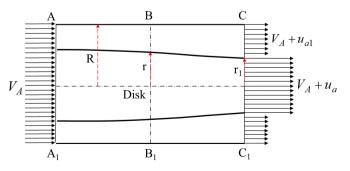
Figure 11. Hydrodynamic model of ideal thruster.
