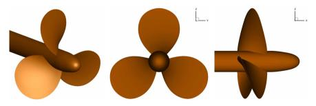
**Figure 1.** Geometry of DTMB 4119 propeller (left: 3D view; middle: front view; right: side view).
