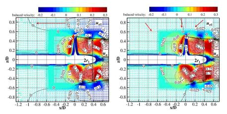
Figure 12. Induced velocity vector distribution (Left: restricted channel; right: open water).
