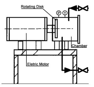
Figure 2. Rotating Disk Device (P symbolizes the manometer and T symbolizes the thermometer).
