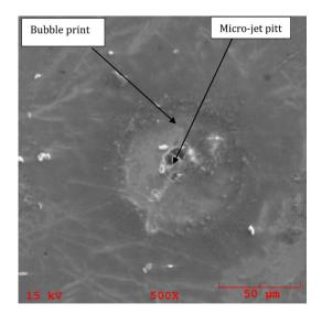
Figure 6. Bubble print on carbon steel test specimen with magnification of 500×.
