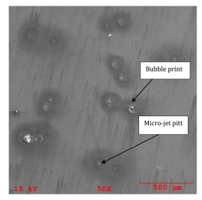
Figure 4. Bubble print on carbon steel test specimen with magnification of 50×.
