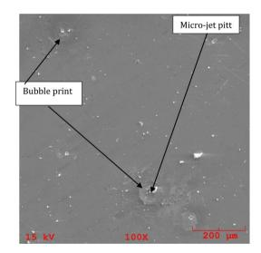
Figure 5. Bubble prints on carbon steel test specimen with magnification of 100×.
