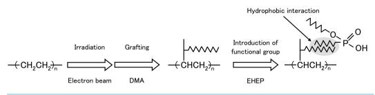
Figure 1. Preparation scheme of graft adsorbent containing EHEP.
