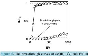
$(\triangle)$  with the mixture solution of Sc(III) and Fe(III) at pH1.
