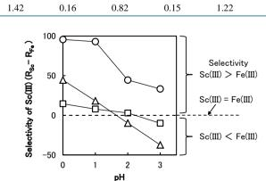
**Figure 4.** Effect of pH on the adsorption selectivity for Sc(III) versus Fe(III) of EHEP ( $\bigcirc$ ), GMA-PA ( $\triangle$ ) and HMPA ( $\Box$ ).
