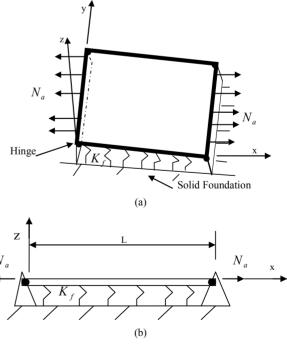
Figure 1. System under consideration. (a) A thin plat on winkler foundation hinged at the two opposite sides and free at the other two sides; (b) The corresponding beam model.
