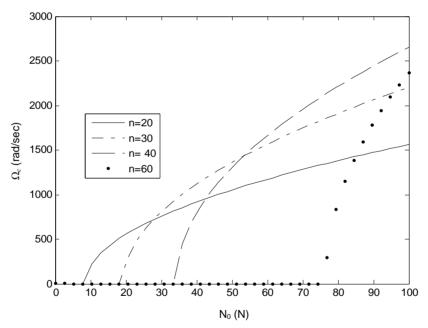
Figure 8. Critical frequency  $\Omega_c$  versus static axial lada  $N_0$  for different values of wrinkles number n.  $K_f = 103 \text{ N/m}^2$ , h = 0.22 mm.
