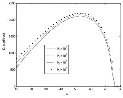
Figure 10. Variation of critical frequency  $\Omega_c$  with number of wrinkles n. h = 0.23 mm,  $N_0 = 50$  N.
