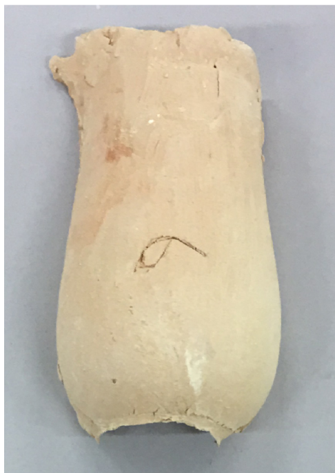
Figure 27. S6 sample, showing clay compaction after firing and notice the shrinking caused body bindi.
