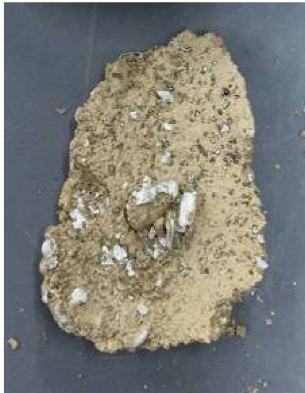
Figure 26. S4 sample showing demolishing and crashing after firing.
