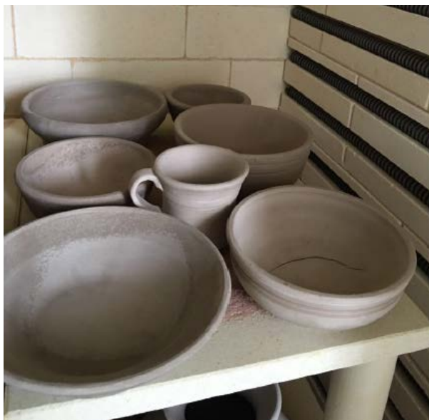
Figure 21. Firing all samples under temperature of 1031 Celsius.
