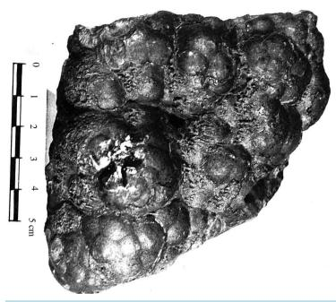
**Figure 10.** A hand specimen of psilomelane showing typical botryoidal or kidney-like form from Jai Bhawani quarry, Garbham, Vizianagram-Visakhapatnam Manganese Belt (A.P.).
