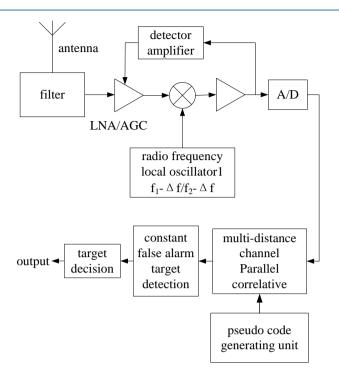
Figure 3. The receiving module of rangefinder.
