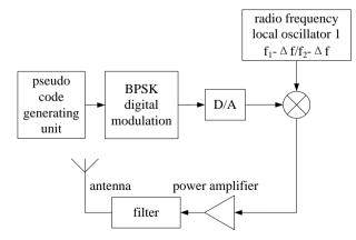
Figure 2. The sending module of rangefinder.
