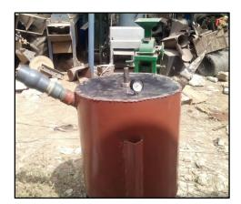
Plate 1. Biogas digester.
