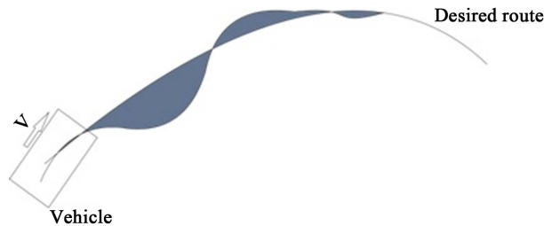
Figure 9. Lateral displacement area.
