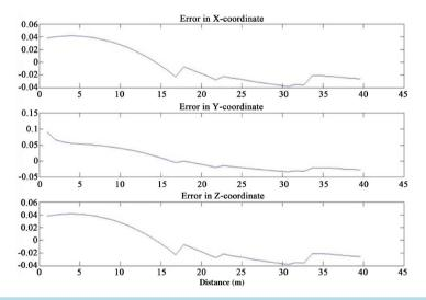
Figure 5. Relative error in the coordinates for a random walk in the calibrated environment. The *x*-axis is the iteration number while the *y*-axis is the relative error in localizing the target using stereovision versus the known simulated coordinate.
