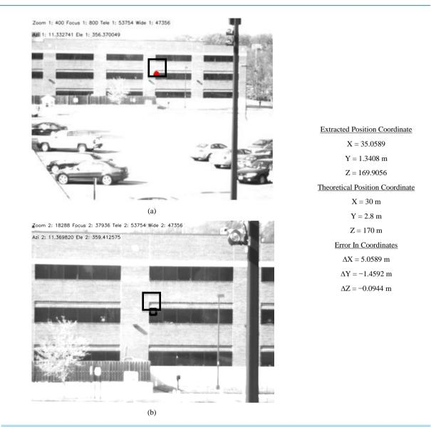
Figure 9. (a) Master Camera looking at a building with its point selected in a box; (b) Slave camera centering that point within its image and computing the position relative to the master camera.
