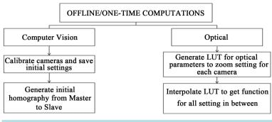
Figure 1. Calibration phase of the surveillance system.
