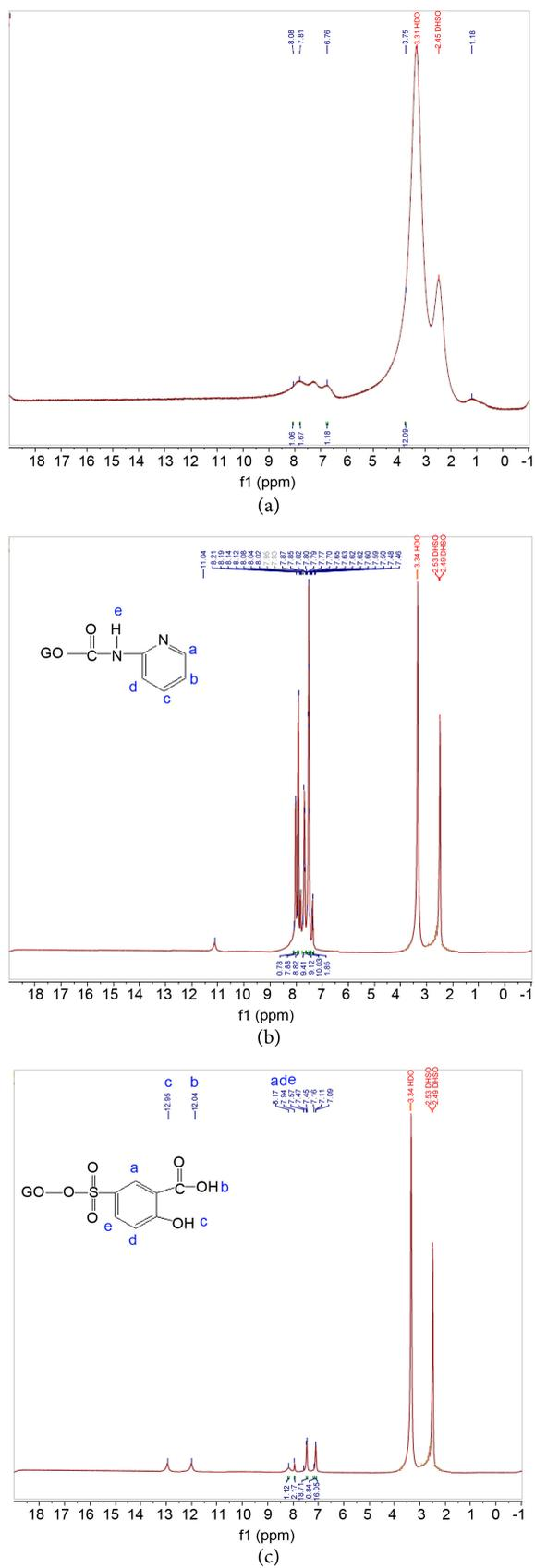
**Figure 5.**  $^1\text{H}$  NMR spectrum of (a) GO (b) GAP (c) GSO.
