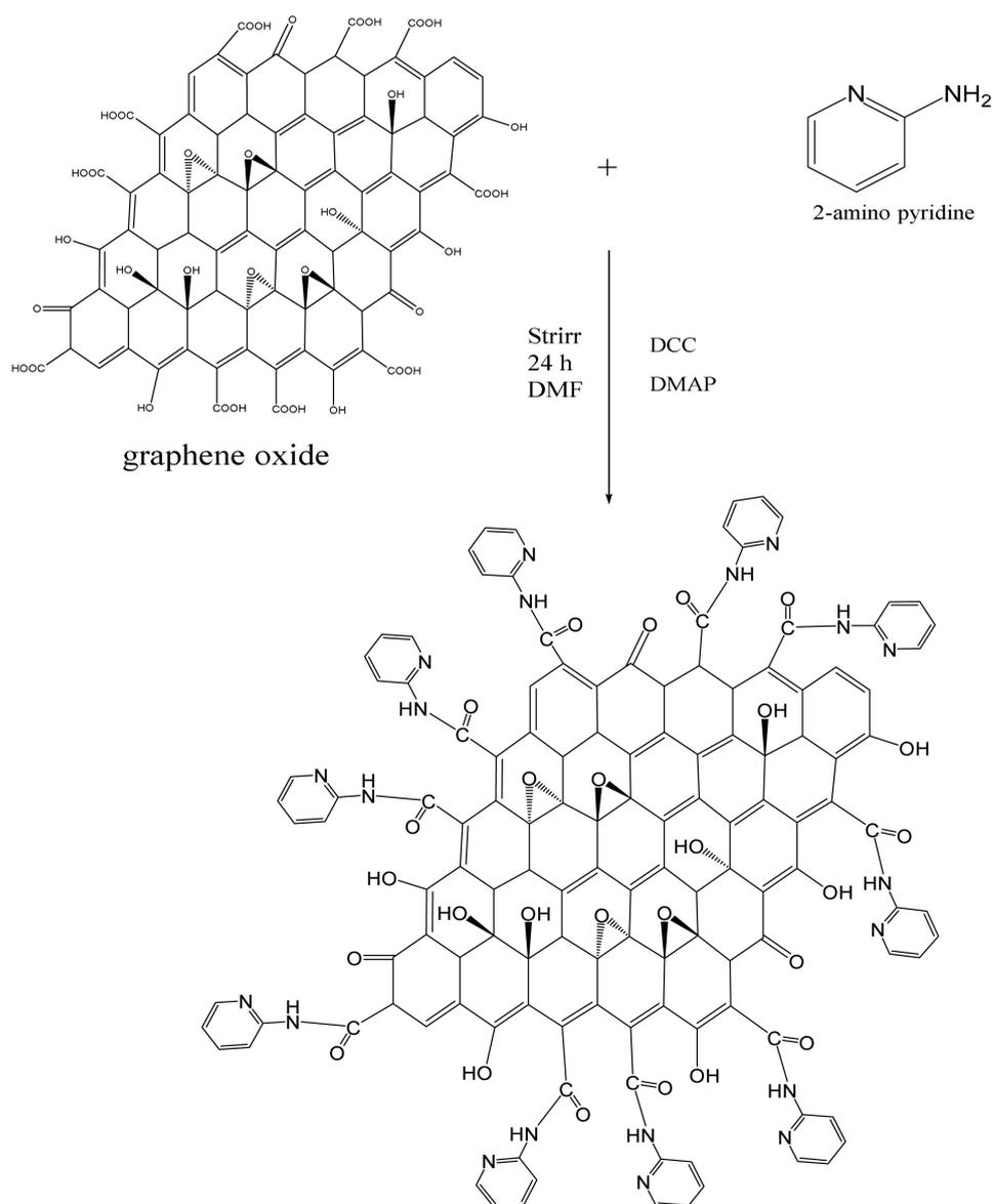
**Figure 2.** Chemical equation of preparation (GAP).
