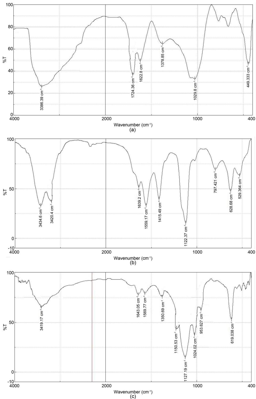
**Figure 4.** FTIR spectrum of (a) GO powder (b) GAP powder (c) GSO powder.
