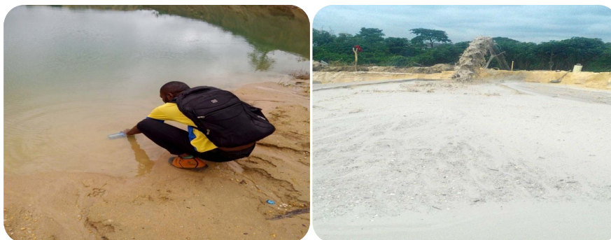
Figure 2. The grab method for water collection and collection of sediment through manual dredging.
