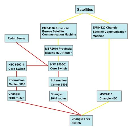
Figure 3. Radar station satellite communication network structure.
