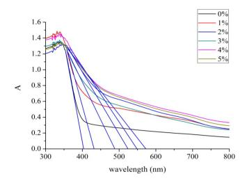
Figure 4. Absorption wavelength of vanadium doped titanium dioxide photocatalyst.
