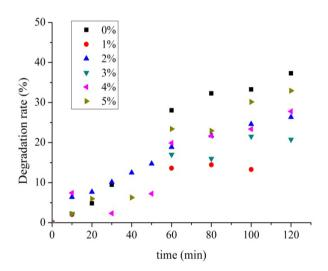
Figure 5. Degradation of SDBS by doped vanadium titanium dioxide photocatalyst.
