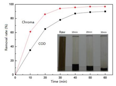
Figure 3. Effect of treatment of washing and dying wastewater with nano flocculant.
