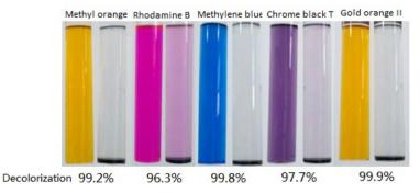
Figure 2. Effect of treatment of simulated dye wastewater with nano flocculant.
