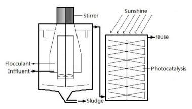
Figure 1. Flow diagram of combined process for washing and dyeing wastewater treatment.
