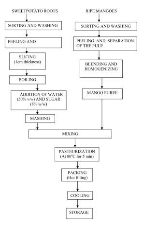
Figure 1. Product manufacture flow diagram.
