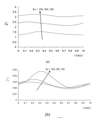
Figure 7. (a) Periodic oscillation of Nu with  $\varepsilon = 0.1$  m/s and  $\tau = 1$  sec; (b) Periodic oscillation of  $\overline{c_f}$  with  $\varepsilon = 0.1$  m/s and  $\tau = 1$  sec.
