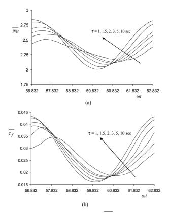
Figure 4. (a) Periodic oscillation of Nu with  $\varepsilon = 0.1$  m/s, and Re = 200; (b) Periodic oscillation of  $\overline{c_f}$  with  $\varepsilon = 0.1$  m/s, and Re = 200.
