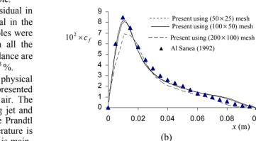
Figure 2. (a) Variation of Nusselt number along the heated plate.Re = 200, h/d = 4, L/d = 20 and Pr = 0.71; (b) Variation of friction coefficient along the heated plate. Re = 200, h/d = 4, L/d = 20 and Pr = 0.71.
