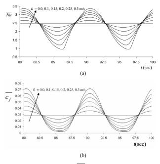
Figure 3. (a) Oscillation of  $\overline{Nu}$  with  $\tau = 10$  sec and Re = 200; (b) Oscillation of  $\overline{c_f}$  with  $\tau = 10$  sec and Re = 200.
