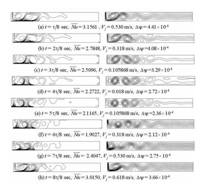
Figure 6. Isotherms,  $\Delta T = 1$ K (left) and streamlines (right) for a cycle of oscillation with  $\varepsilon = 0.3$  m/s,  $\tau = 2$  sec, and Re= 200.
