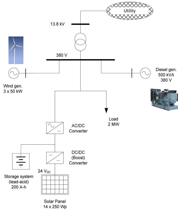
**Figure 1.** Components of the commercial building used in the analysis.
