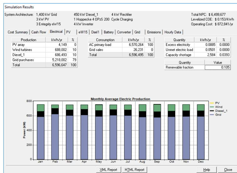
Figure 5. Power supply from the utility and the local sources of the building (Case 2).
