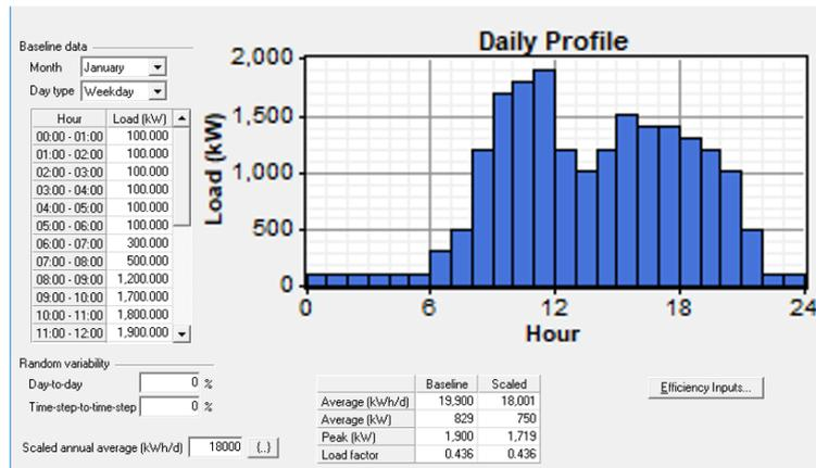
Figure 4. Details of the load curve (Case 2).
