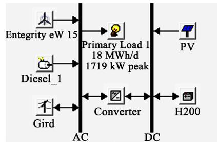
**Figure 3.** Load fed by the utility and the sources of the building.
