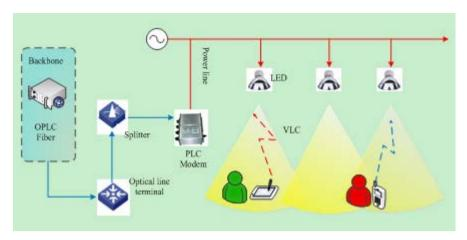
Figure 2. The network architecture VLC-PLC depth integrated communication.
