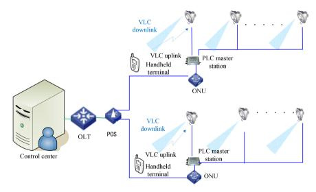
Figure 3. The sketch of intelligent network structure of substation or cable tunnel.
