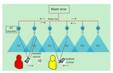
Figure 4. The diagram of hybrid VLC-PLC system service.
