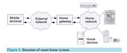
visual interface. In this system, the home server and ZigBee coordinator constitute the home gateway together, which is responsible for connecting the external network and the internal network. The home server communicates with the coordinator through the serial port. At the same time, the home server is connected to the mobile terminal through the external network, and transfers data to the mobile terminal through the Socket communication.
