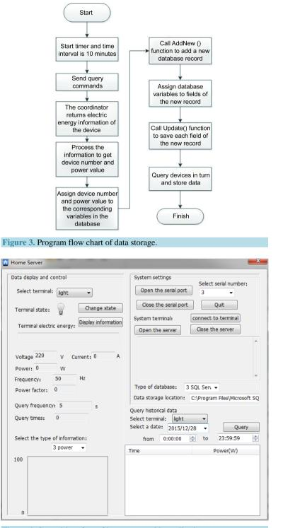
Figure 4. Control interface of home server-side application.
