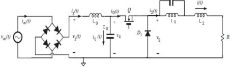
Figure 3. A proposed converter with parallel net.
