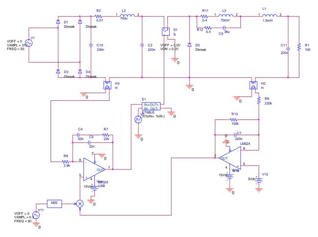
Figure 8. Pspice simulation block.
