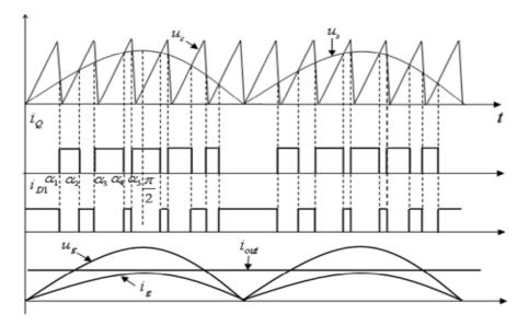
Figure 7. Waveforms of proposed converters:  $u_s$ —modulating wave;  $u_c$ —carrier wave;  $i_Q$ —switch current;  $i_{D1}$ —diode current.
