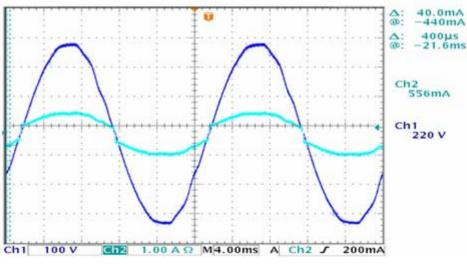
(a) Input voltage: 220V (RMS); Input current: 550mA (RMS) load: 100 $\Omega$ ; Power factor: 0.974
