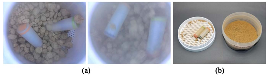
Figure 6. Case when clods and two rods were combined in jar: (a) Process of stirring; and (b) result after two minutes of stirring.
