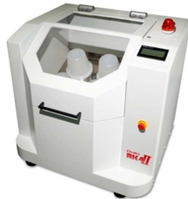
Figure 1. Rod mill (DIK-2610, Daiki Co.), which operates without release of soil dust into the surroundings and functions to transform the median size of soil particles to be <2-mm diam.
