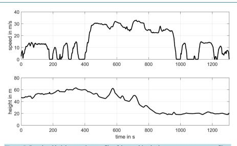
Figure 5. Speed and height over time profile of the combined urban motorway usage profile.
