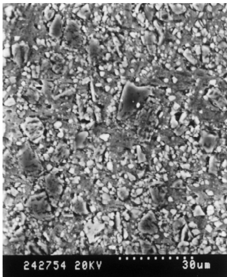
Figure 1. Microstructure of aluminum matrix composite SiC p /A356.
