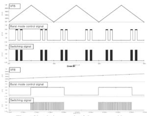
Fig. 6 Simulation result of the proposed burst mode control circuit
