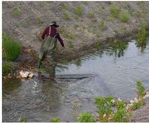
Figure 3. Velocity measurement around the drop structure.
