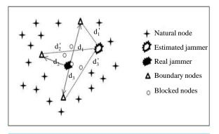
Figure 3. Estimation of jammer localization.
