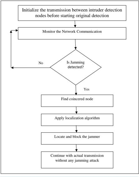
Figure 2. The proposed framework flowchart.
