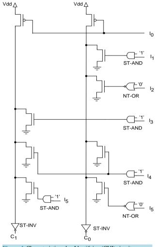
Figure 4. Characteristic value Identifying (CVI) circuit.
