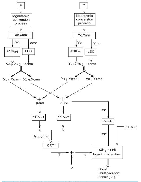
Figure 1. TVL based multiplication process for RLNS based system
