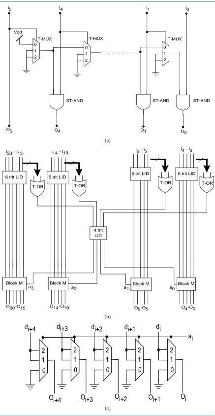
Figure 3. (a) Leading trit detecting (LTD) circuit; (b) 21 trit LID circuit; (c) Block M.
