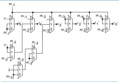
Figure 7. Antilogarithmic error correction circuit (ALEC) for  $N_t = 6$ .
