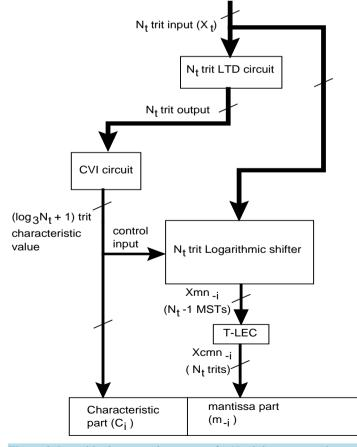
Figure 2. Logarithmic conversion process for N<sub>t</sub> trit input operand.
