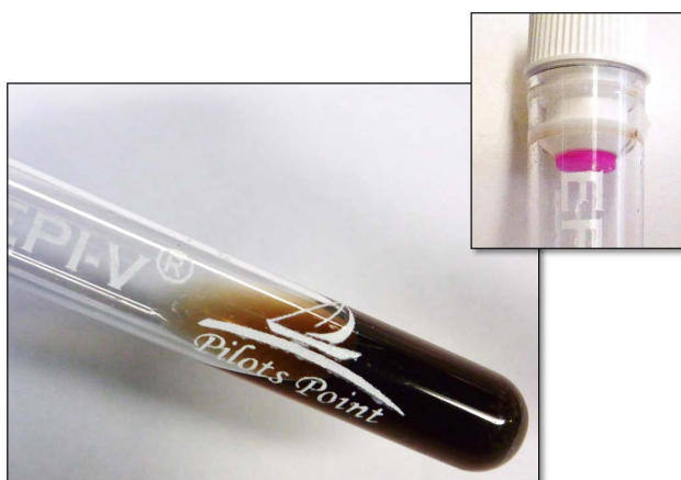
Figure 2. Positive EPI-V ® . Positive EPI-V ® liquid is dark brown-black and the disk in the cap is bright fuchsia.
