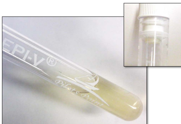
Figure 1. Negative EPI-V ® . Negative EPI-V ® liquid is straw-colored and the disk in the cap is white.
