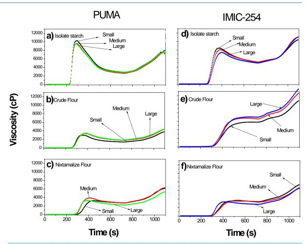
Figure 7. A to F shows the pasting profiles of isolated starches, the crude maize flours, as well as nixtamalized maize flours obtained from small, medium and large Puma and IMIC-254 grains as a function of the time.
