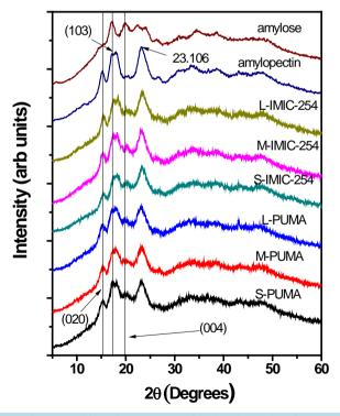
**Figure 6.** X-ray diffraction patterns of isolated starches from small, medium, and large maize grains for IMIC-254 and Puma, as well as amylopectin and amylose from Sigma Aldrich taken as reference.
