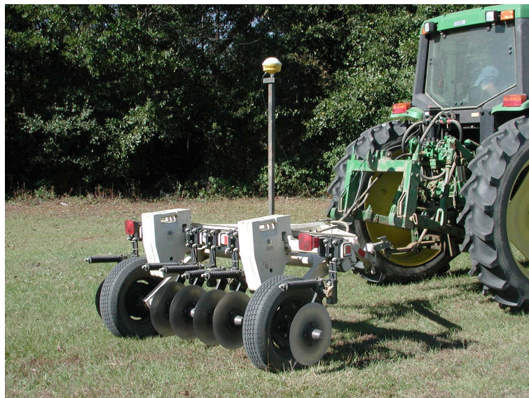
Figure 1. The Veris 3100 soil electrical conductivity meter.
