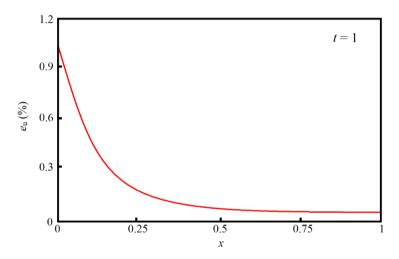
**Figure 2.** Depiction of discrepancy (*i.e.*, error) between the present iterative method and exact solution due to Equation (22).
