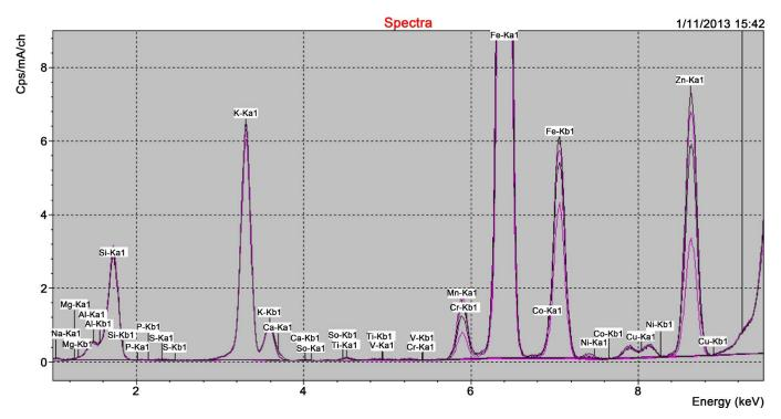
**Figure 4.** Head and tail spectra in energy range 1 to 9.5 keV. Here spectra of leached tails from three different exposure times using 4% sulfuric acid on 2 - 4 mm particles are compared to the head sample, the upper black curve. Upper red curve is 1 day, lower black curve 5 days, and lower red curve 2 weeks. Increasing dissolution of such undesirable gangue metals as Mn, Fe, and Zn with increased leach time is evident.
