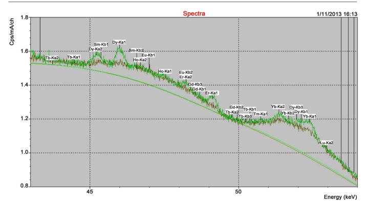
Figure 3. Head and tail spectra in energy range 43 to 54 keV. Near complete ("flatline") recoveries of 80% - 90% are evident for such target, high value HREEs as Dy and Yb.
