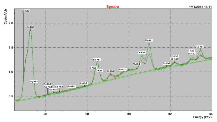
**Figure 1.** Head (green) and post-leach tail (black) XRF spectra in the energy window from 24 to 34 keV (x-axis). Peak height (y-axis) is recorded X-ray counts per second (Cps) per milliamp (mA) per channel (16,000-channel analyzer). Difference between head and tail curve is portion of target element extracted into leach solution. Note small difference between head and tail for Sn (little extraction), versus significant differences for Cs and La.
