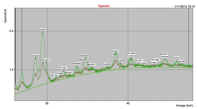
Figure 2. Head and tail spectra in energy range 33 to 44 keV. In this sample, significant recoveries are seen for the light REEs. By visual estimate, Ce, at left, has about 55% recovery, and Nd, Sm, and Gd about 65% recoveries.
