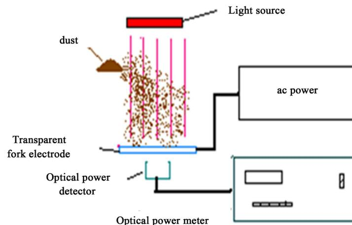
**Figure 1.** Schematic diagram of dust removal experiment device.
