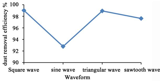
Figure 2. Impact of waveform on dust removal efficiency.
