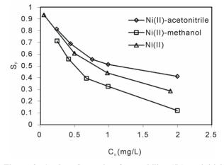
Figure 2. A plot of sorption favourability  $(S_F)$  vs initial metal ion concentration for the removal of Ni(II) ions by alginate-*E. crassipes* beads. pH 4.0, T = 30°C ± 0.2°C, agitation rate = 150 rpm, t = 3 hr, C<sub>0</sub> = 0.05 - 2 mg/L, biosorbent dose = 4 g/L.
