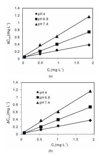
Figure 3. Plots of  $\Delta C_{ads}$  against initial metal concentration for the adsorption of (a) Ni(II) and (b) Ni(II)-TAN onto alginate-*E. crassipes* beads. pH 4.0, T = 30°C ± 0.2°C, agitation rate = 150 rpm, *t* = 3 hr, C<sub>0</sub> = 0.05 - 2 mg/L, biosorbent dose = 4 g/L.
