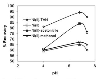
Figure 5. Effect of pH on the recovery of Ni(II) in the presence and absence of TAN, methanol and acetonitrile.
