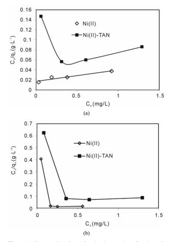
Figure 1. Langmuir adsorption isotherm plots for the adsorption of Ni(II) onto alginate-*E. crassipes* beads in the presence and absence of TAN. (a) pH 4, (b) pH 6.8.
