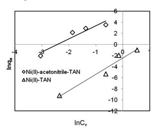
Figure 4. Freundlich adsorption isotherms for Ni(II)-TAN and Ni(II)-acetonitrile-TAN onto alginate-*E. crassipes* beads. pH 4.0, T =  $30^{\circ}$ C  $\pm$  0.2 °C, agitation rate = 150 rpm, *t* = 3 hr, C<sub>0</sub> = 0.05 - 2 mg/L, biosorbent dose = 4 g/L.
