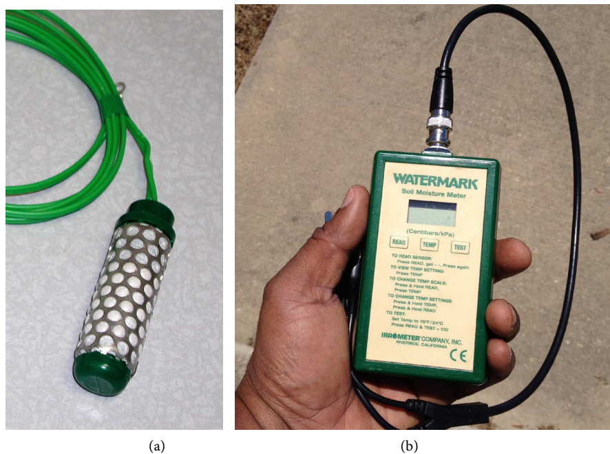
Figure 1. (a) Watermark 200SS sensor; (b) Watermark 200SS manual readout.
