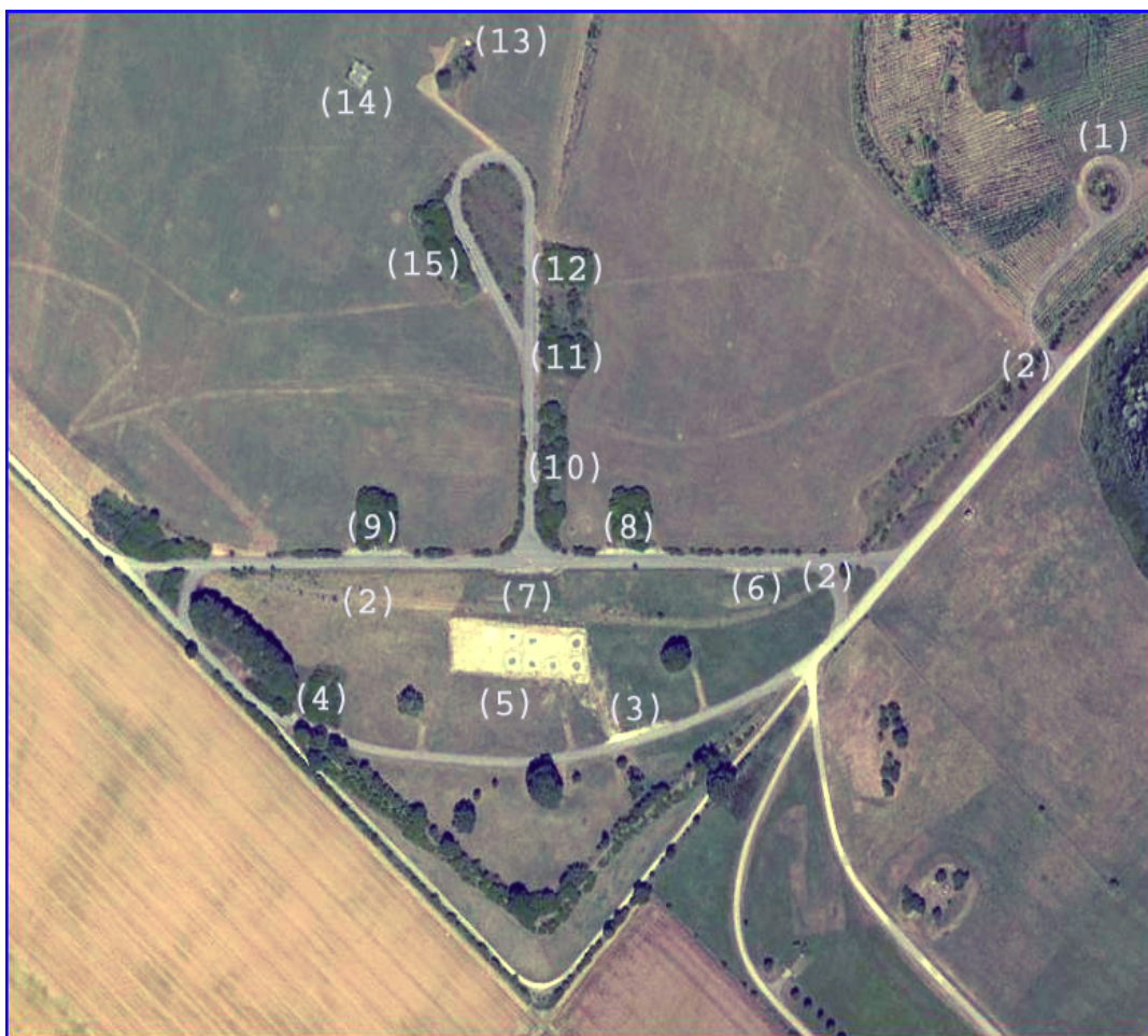
Figure 9. Airfield fuel area—(1) circular structure of unknown purpose, (2) railway, (3)-(4) underground cisterns coded 1, 2, (5) rectangular structure, (6) underground cistern coded 5, (7) underground cistern, (8) underground cistern coded 6, (9) underground cistern coded 7, (10) underground cisterns coded 8, 9, (11) underground cistern coded 10, (12) underground cistern, (13) small underground cisterns, (14) square structure, (15) underground cisterns coded 12, 13.
