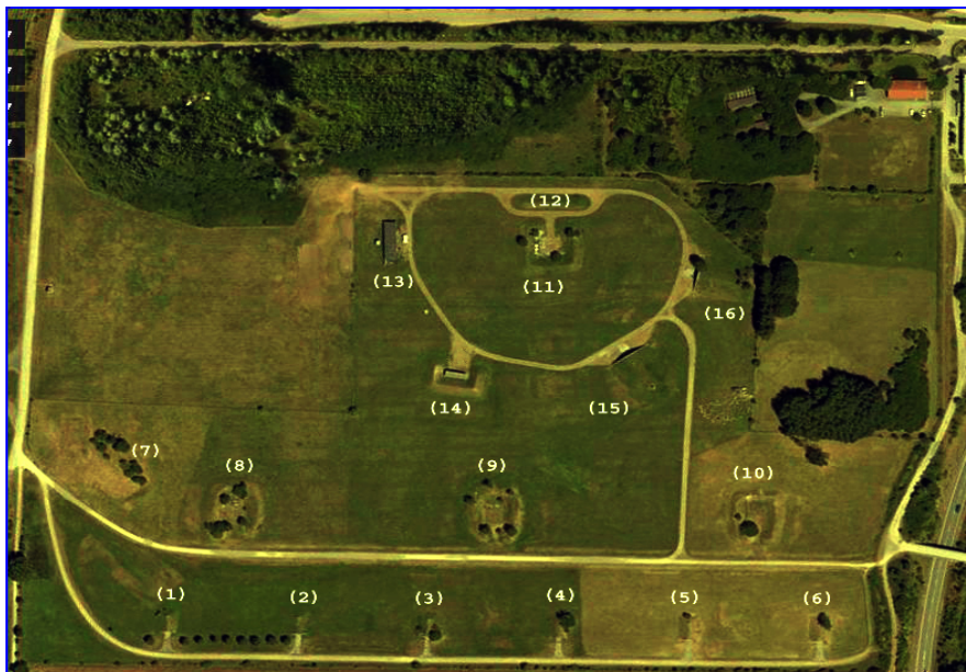
Figure 18. Airfield ammunition area: (1)-(6) ammunition bunkers coded 133, 127, 128, 120, 130, 131; airfield defense area: (7) protection embankment, (8)-(11) gun emplacements, (12) protection embankment, (13) barrack, (14)-(16) bunkers.
