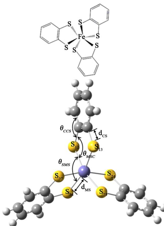
**Figure 2.** Metal binding to benzene-1,2-dithiolate, optimized geometry of the  $[\text{Fe}(\text{bdt})_3]^{3-}$  complex.
