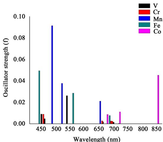
**Figure 4.** UV-vis spectrum of the tris  $[M(\text{bdt})_3]^{3-}$  ( $M = \text{V to Co}$ ) complexes obtained from the present calculation.
